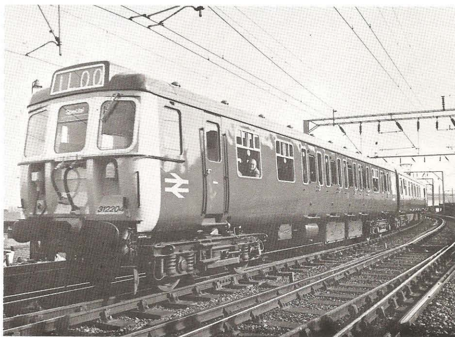
Fig 1. British Railways Class 312 suburban electric multiple-unit for longer distance services made up in four-car sets
